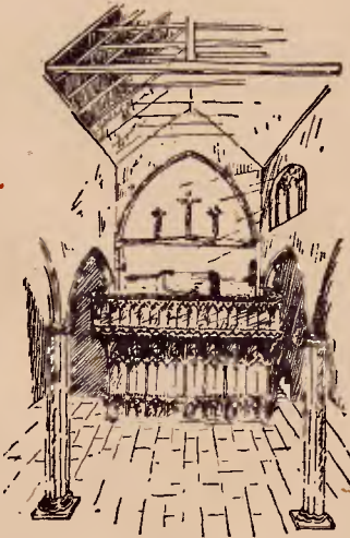
Fig. 5.—Rood loft with rood screen below; rood beam and rood above; rood stairs at side; rood window high up on right side.
