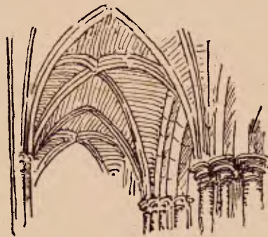
Fig. 2.—Pointed Vaulting with moulded ribs.
